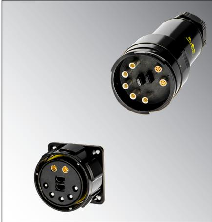
**LKO 32T12M12S2E:** 2 Gigabit contacts, 5 pins size 8, 2 MTP fibre connectors.
